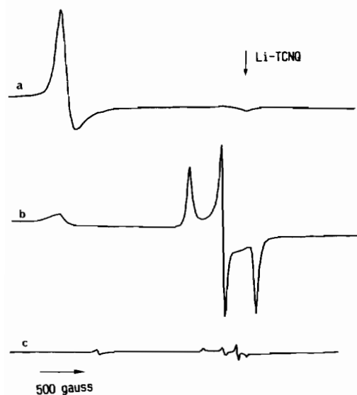
Fig. 2. ESR spectra observed at 77 K for the same reaction solution supplied for optical measurements at 298 K (Fig. 1(a) to (c)): (a) ESR spectrum observed for DMSO solution of Fe(III)TPPCl (0.5 mM, 0.4 ml); (b) ESR spectrum observed after addition of sodium methoxide methanol solution (0.75 M, 0.012 ml); (c) spectrum observed after addition of n-BHPO (1.0 M, 0.02 ml) to the reaction mixture of (b) at 298 K.
